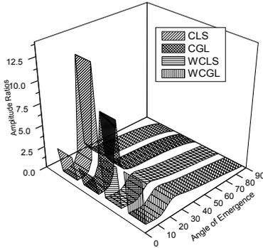
**Fig.17** Variation of amplitude ratios of transmitted SV2-waves versus angle of incidence.
