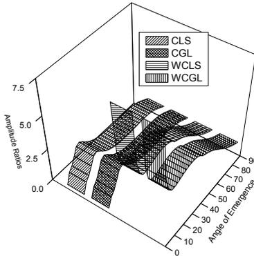
**Fig.2** Variation of amplitude ratios of reflected P-waves versus angle of incidence.
