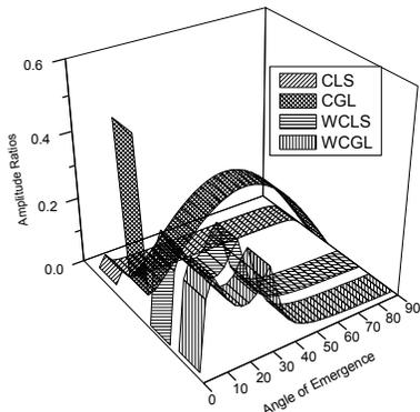
**Fig.18** Variation of amplitude ratios of reflected P-waves versus angle of incidence.
