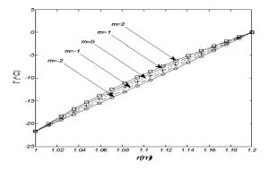
Fig. 2 Temperature distribution of radial at  $\theta = \pi / 3$ .
