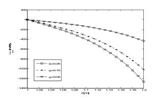
**Fig. 15**Hoop thermal stress in the cross section of cylindrical based on the compressibility coefficient (*B*) changing.
