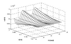
$\label{eq:Fig.3} \textbf{Radial displacement in the cross section of cylindrical}.$
