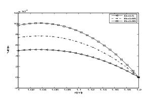
Fig. 21 Circumferential displacement in the cross section of cylindrical based on the compressibility coefficient (*B*) changing.
