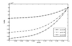
Fig. 40 Radial displacement in the cross section of cylindrical based on the pore volume fraction  $(\phi)$  changing.
