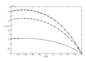
Fig. 22 Circumferential displacement in the cross section of cylindrical based on the pore volume fraction  $(\phi)$  changing.
