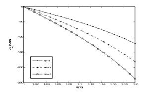
Shear distribution of radial thermal stress  $\sigma_{r\theta}$  at  $\theta = \pi/3$ .
