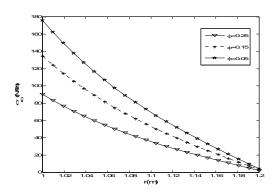
Fig. 38 Shear thermal stress in the cross section of cylindrical based on the pore volume fraction  $(\phi)$  changing.
