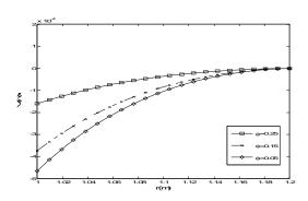
Fig. 42 Circumferential displacement in the cross section of cylindrical based on the pore volume fraction  $(\phi)$  changing.
