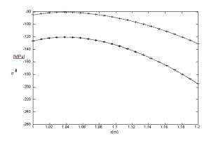
Fig.30 Hoop distribution of radial thermal stress  $\sigma_{\theta\theta}$  at  $\,\theta=\pi$  / 3.
