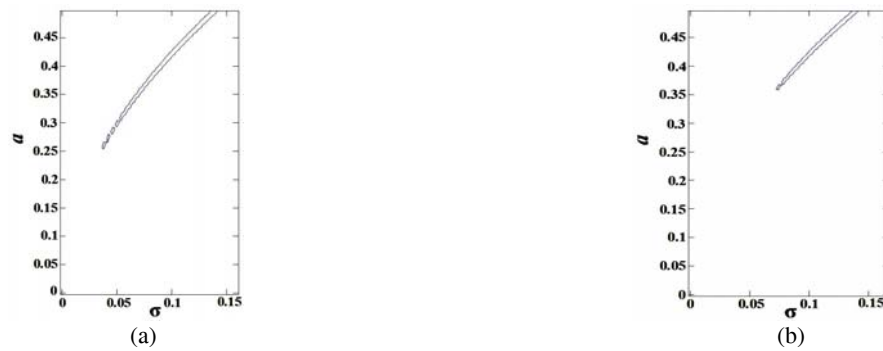
Fig. 9 Effects of \mu on the amplitude for \eta = 0.5, \lambda = 1, P = 0.1, \beta = 3 , (a) \mu = 0.0002 , (b) \mu = 0.001 .
