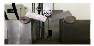
**Fig.6** The three-point bending test device during the test.
