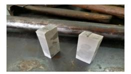
Fig.7 A sample that was broken after taking out from liquid nitrogen.
