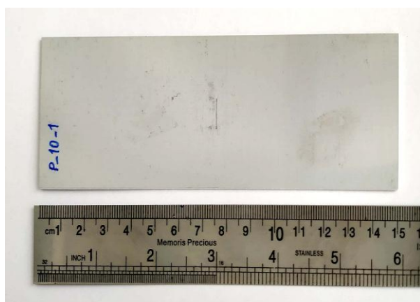
Fig.9 Sample with 10 mm crack.
