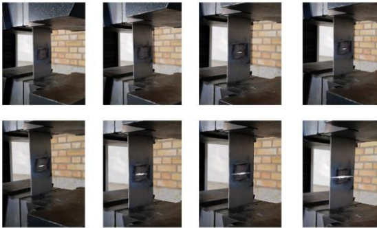
Fig.12 Crack propagation stages of repaired piece.
