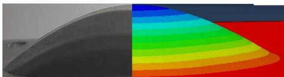
**Fig.9** Displacement profile in  $z$  direction for  $15^\circ$ .
