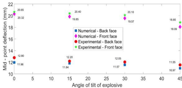
**Fig.8** Comparison between central numerical and experimental of back face sheet deflection.
