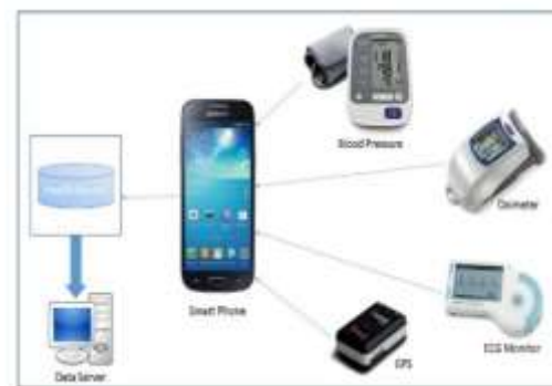
Fig. 2. Patient monitoring system using smart phones.
