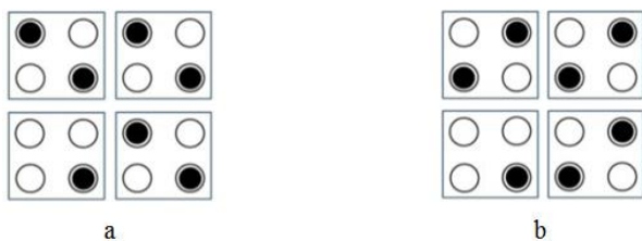
Fig. 5. Two cases for fault occurrence and influence of defective cell on the output logic. (a) The faulty cell in the lower binary wire and the logic level '0' for the upper binary wire will polarize the next cells to logic level '0'. (b) The faulty cell in the lower binary wire and the logic level '1' for the upper binary wire will polarize the next cells to logic level '1'.
