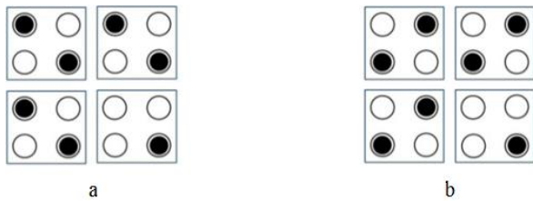
Fig. 4. Electron position in case of lower defective cell. (a) Previous cell with logic level '0' with the faulty cell in the lower binary wire and the single electron in position 2. (b) Previous cell with logic level '1' with the faulty cell in the lower binary wire and the single electron in position 2
