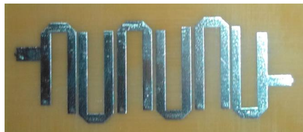
Fig. 7. Implemented (Fabricated) Hairpin Filter
