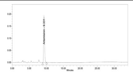
Fig. 3. HPLC chromatogram of artemisinin standard showing a single major peak at 9.331 min.
