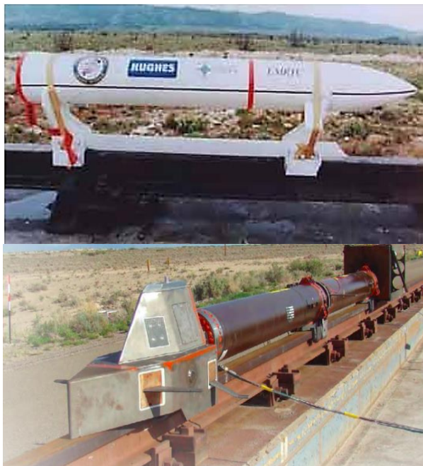
Fig. 2 Real example of mono-rail sled system [8].
