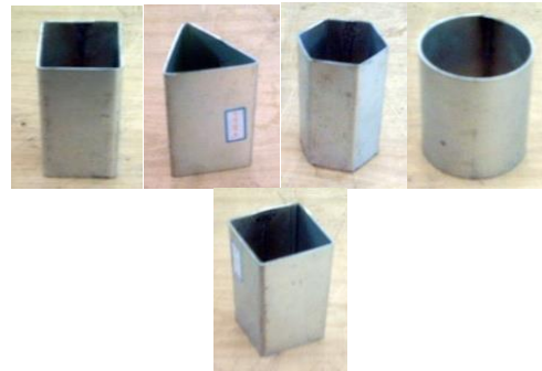
Fig. 2 Prepared specimens with various section geometries.
