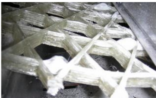
Fig. 8 Fiber buckling in the upside layers of the panel.
