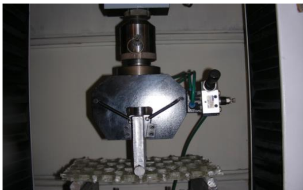
Fig. 4 Three-point bending test of composite grid panel.
