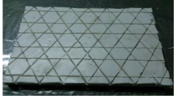
Fig. 3 Silicon rubber mold.
