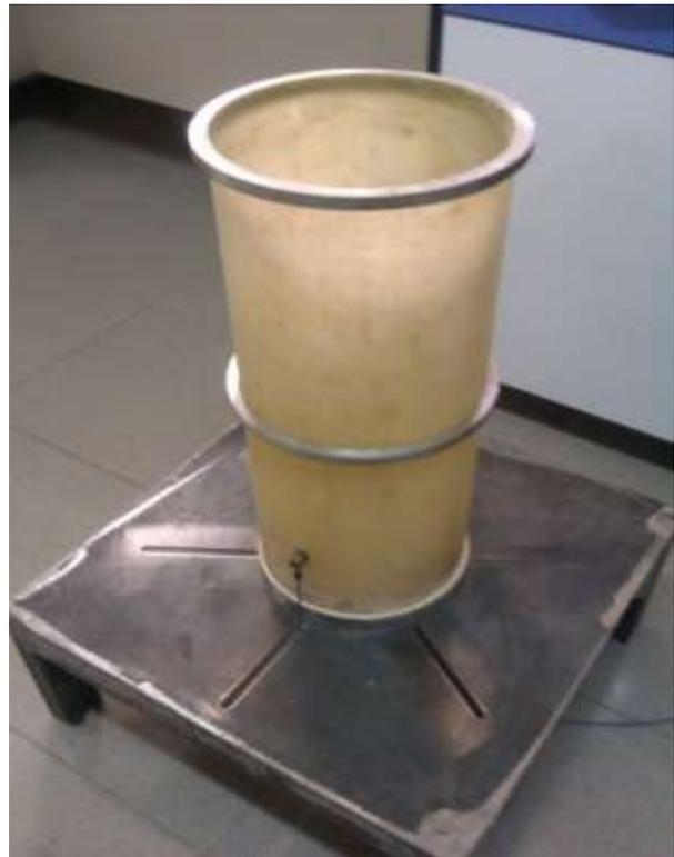
**Fig. 4** Ring-stiffened clamped-free composite cylindrical shell
