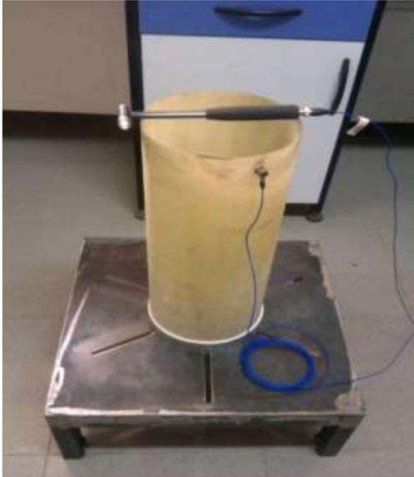
**Fig. 2** Clamped-free composite cylindrical shell with hammer and piezoelectric accelerometer.
