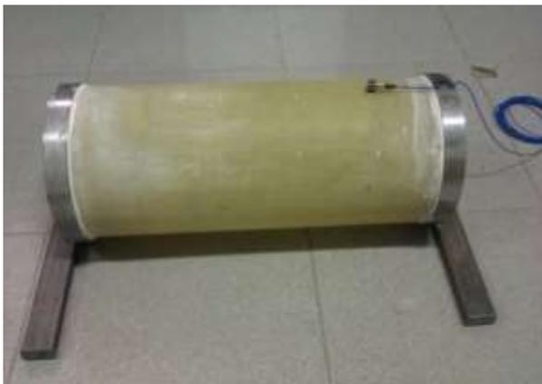
**Fig. 3** Clamped-clamped composite cylindrical shell.
