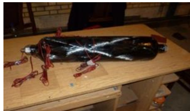
Fig. 13 Vessel after Filament Winding.
