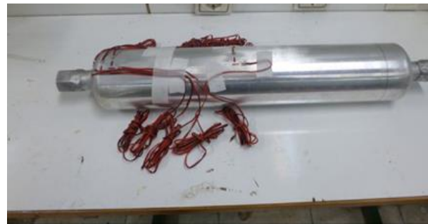
Fig. 12 Liner Vessel After Strain Gauge Installation.
