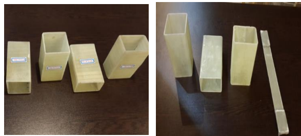
(a): with wires (b): without wires Fig. 1 Composite tubes with different cross sections.
