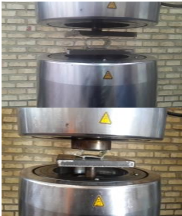
Fig. 4 Square composite tube before and after lateral loading.
