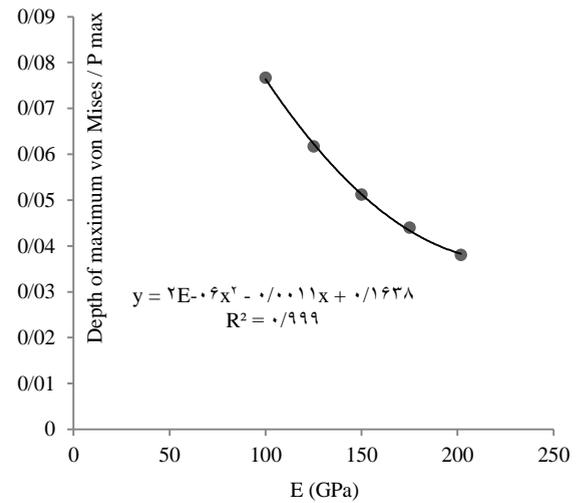
Fig. 7 The ratio of depth of maximum von Mises stress to maximum contact pressure vs. elastic modulus.
