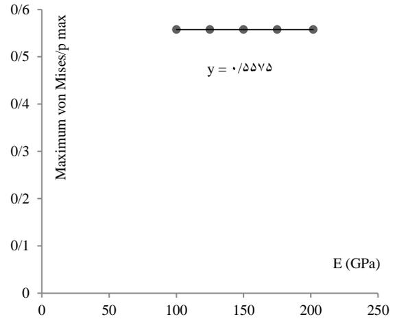
Fig. 6 The ratio of maximum von Mises stress to maximum contact pressure vs. elastic modulus.
