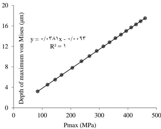
Fig. 5 Variation of the depth of maximum von Mises stress vs. the maximum contact pressure.
