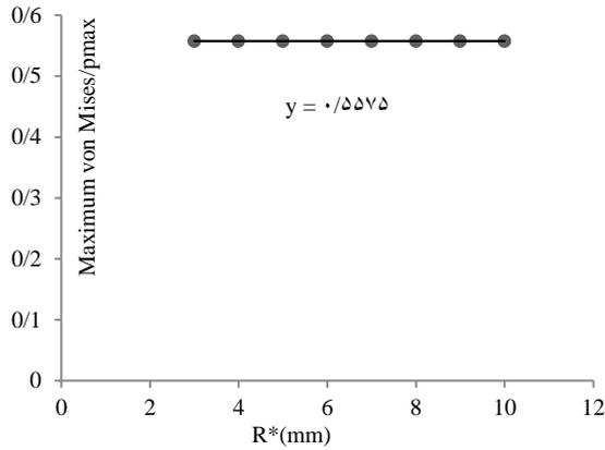
**Fig. 8** The ratio of the maximum von Mises stress to the maximum contact pressure vs. equivalent curvature radius.
