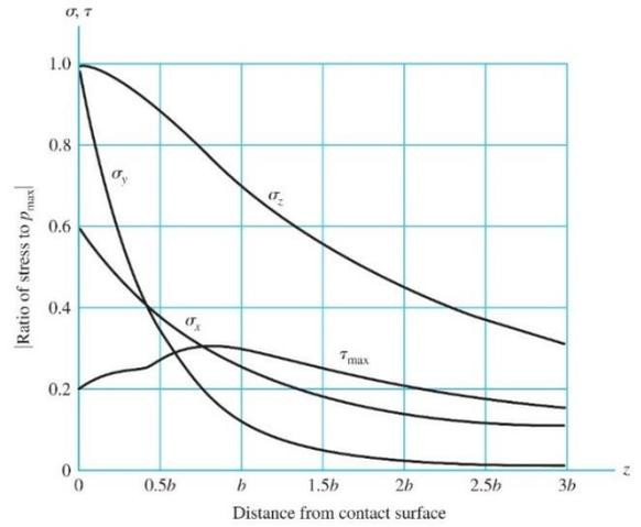
**Fig. 3** Stress components as functions of depth below the contact area [20].
