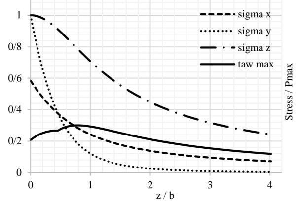
**Fig. 2** Stress components as functions of depth below the contact area.
