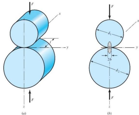
Fig. 1 (a): Two right circular cylinders held in contact by forces  $F$  uniformly distributed along cylinder length  $l$ , and (b): Contact stress has an elliptical distribution across the contact zone width  $2b$  [20].
