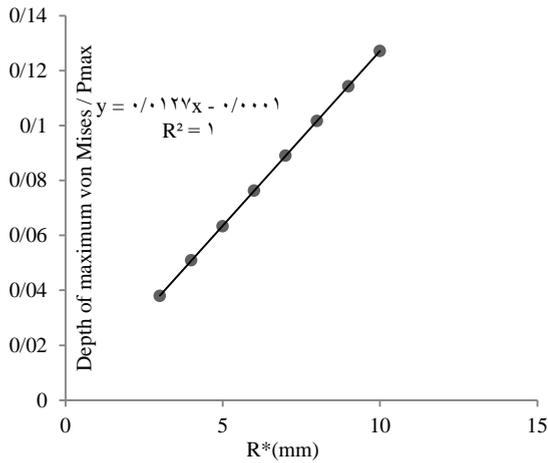
**Fig. 9** The ratio of the depth of maximum von Mises stress to the maximum contact pressure vs. equivalent curvature radius.
