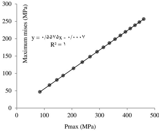
Fig. 4 Variation of the maximum von Mises stress vs. the maximum contact pressure.
