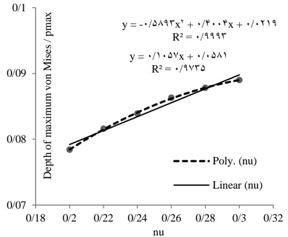
**Fig. 11** The ratio of the depth of maximum von Mises stress to maximum contact pressure vs. Poisson’s ratio.
