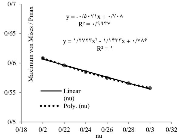
**Fig. 10** The ratio of maximum von Mises stress to maximum contact pressure vs. Poisson’s ratio.
