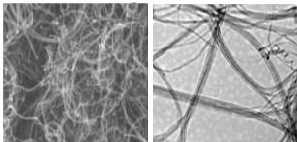
**Fig. 5** SEM and TEM images of the single wall nano carbon tube (SWCNTs).
