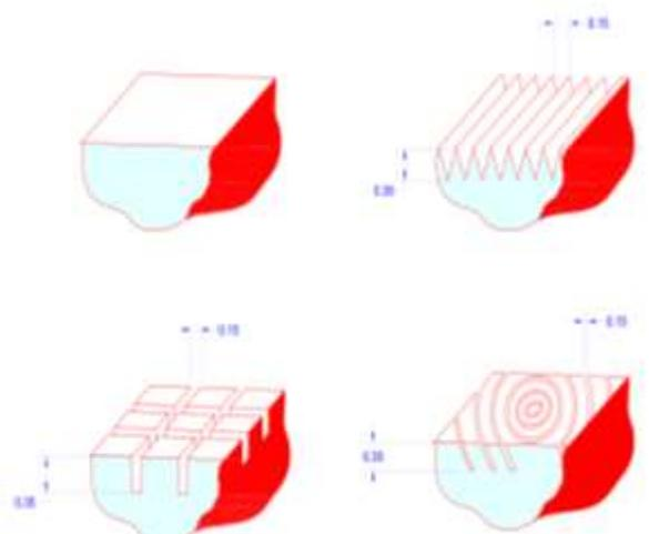
Fig. 4 Schematic of smooth (S0) and grooved surfaces (S1, S2, S3).
