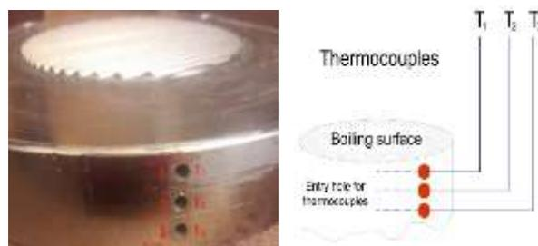
**Fig. 7** (a): Experimental setup of the surface and (B): Boiling surface with three thermocouples embedded inside it.
