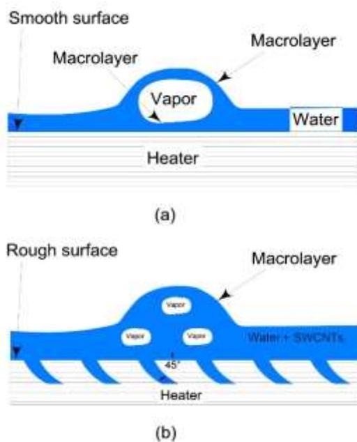
Fig. 12 Schematic of hypothesis for water film structure in pool boiling: (a): with smooth surface and (b): new illustration for vapors formation with groove surface (S3) and nano.
