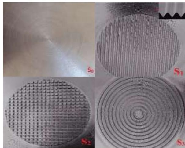
Fig. 3 Various surfaces including smooth (S0) and grooved surfaces (S1, S2, S3).
