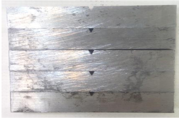
Fig. 2 A group of 5 Charpy samples before failure.
