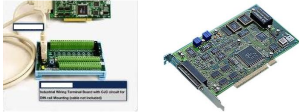
Fig. 9 Data card, external electronic board and the cable
