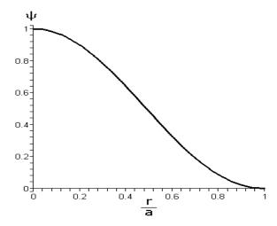
Fig. 3 Dimensionless deflection for clamped plate
