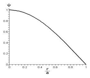
Fig. 2 Dimensionless deflection for pinned plate
