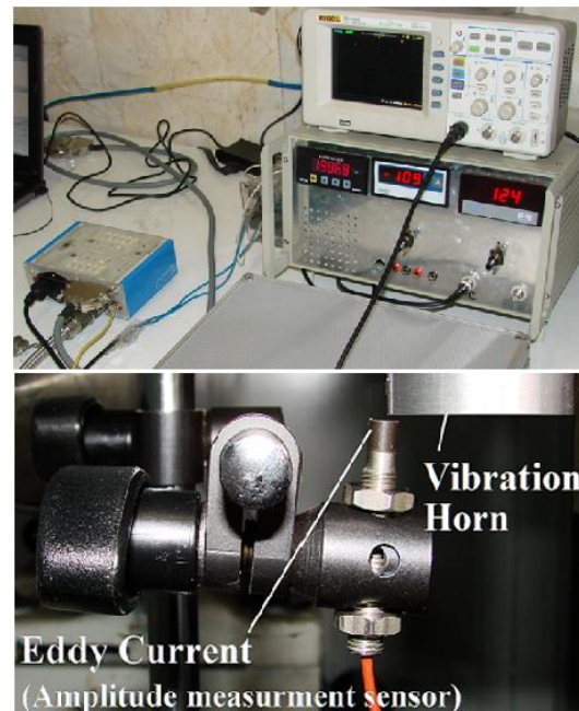
Fig. 5 Ultrasonic generator, Force and amplitude measurement equipment (load cell, data acquisition setup, eddy current and oscilloscope)
