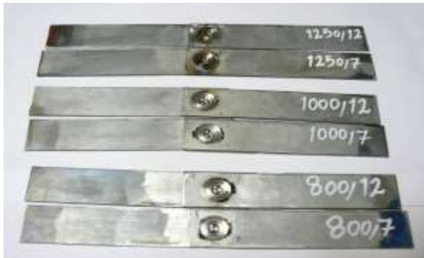
Fig. 5 Images of the welded joints without any defects
