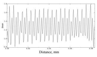
Fig. 9 Variation of PEEQ in the center line of the workpiece after the fourth pressing step
