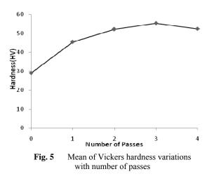
After the second ( $\varepsilon_{eff} = 2.32$ ) and the third ( $\varepsilon_{eff} = 3.48$ ) passes the hardness value increased slightly and then decreased to 47 HV after the fourth pass ( $\varepsilon_{eff} = 4.64$ ) (Fig. 5). The decrease in hardness in subsequent groove pressing step may be due to strain softening after imposing 3.48 strain.
