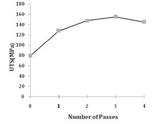
Fig. 7 Ultimate tensile strength against number of passes
