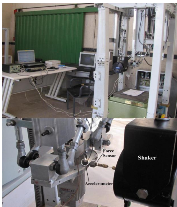
Fig. 5 Modal test of parallel mechanism
