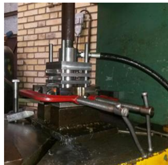
Fig. 2 The die components installed on a hydraulic press unit
