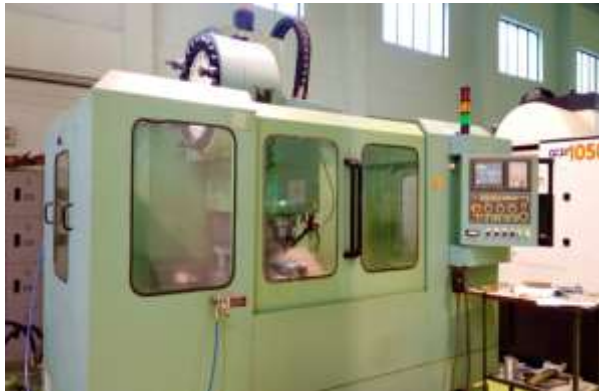
Fig. 2 3-Axis CNC machine used for machining of the Blade
