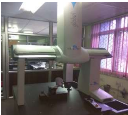
Fig. 11 CMM Global to check deformation
