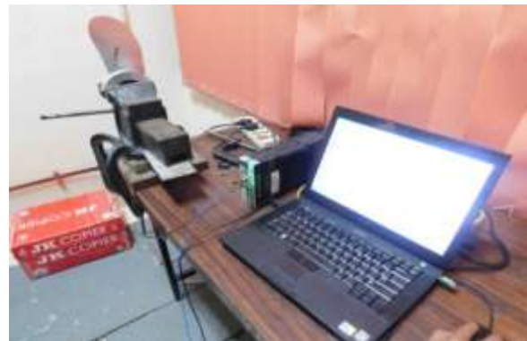
Fig. 13 Experimental setup for impact hammer test method
