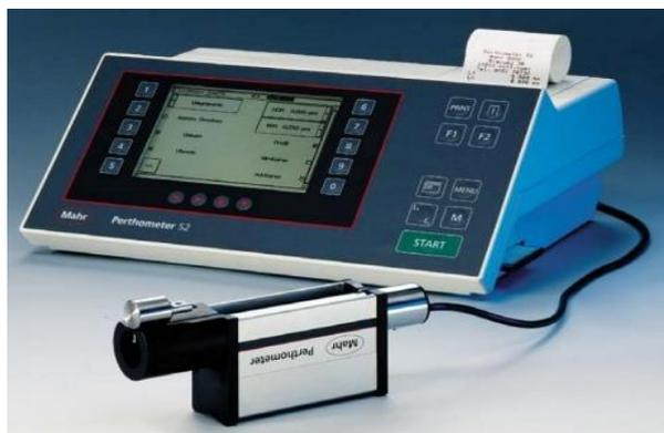
**Fig. 1** Mahr-Perthometer M1 surface roughness tester
