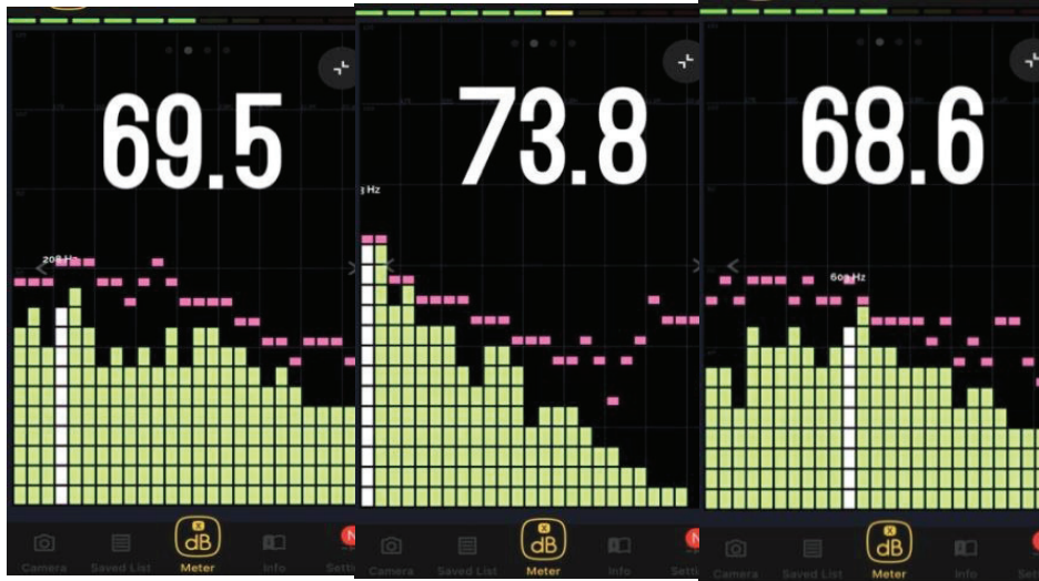
Fig 6. A few samples of sound level (dBA) SPL in the study areas
