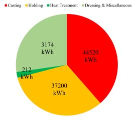
Fig. 3. Foundry Process Steps Energy Consumption (Electricity) October 2016.
