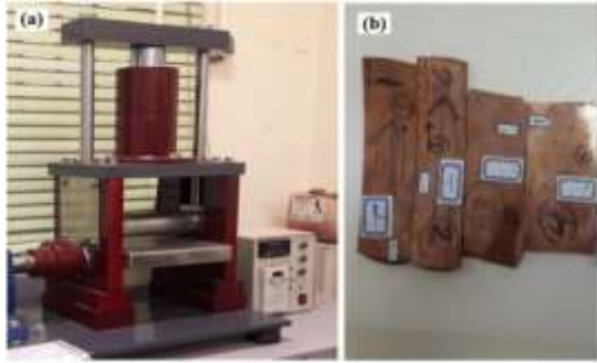
Fig. 3. (a) The rolling machine used and (b) the rolled specimens.
