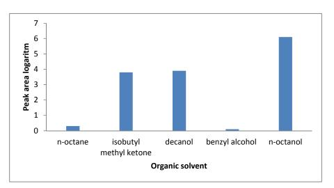
Figure 2. The effect of organic solvent on extraction efficiency of fexofenadine.
