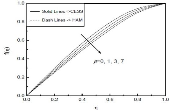
**Figure 6:** Axial velocity curves for different values of  $\beta$  when  $R = 15$ .
