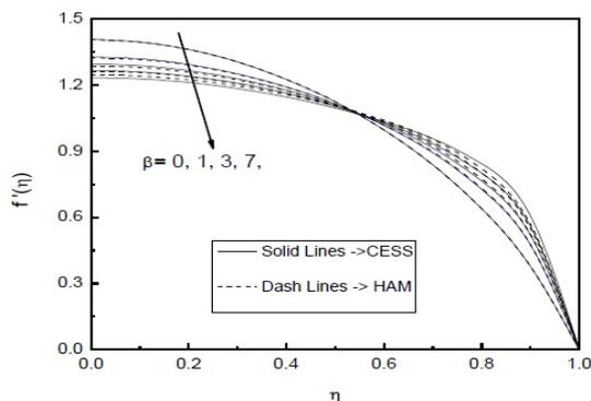
**Figure 7:** Axial velocity curves for different values of  $\beta$  when  $R = 15$ .
