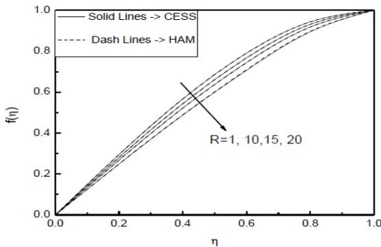
**Figure 4:** Axial velocity curves for different values of  $R$  when  $\beta = 2$ .
