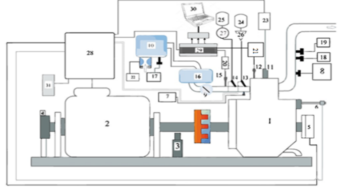
Figure 2: Test platform, control assembly, and measurement systems 1: Engine, 2:dynamometer, 3: engine speed sensor, 4: torque sensor, 5: shaft encoder, 6: suction TDC sensor, 7: inlet mixture temperature sensor,8. exhaust gas temperature sensor, 9: throttle, 10: primary air comfort chamber, 11: spark plug, 12: dynamic pressure transducer, 13: NG injector, 14: gasoline injector, 15: absolute pressure transducer, 16:secondary air comfort chamber, 17:primary comfort tank temperature sensor, 18: gas analyzer a, 19: gas analyzer b, 20: amplifier of the absolute pressure transducer, 21: amplifier of dynamic pressure transducer, 22: inlet air flow sensor, 23: ignition system, 24: NG tank,25: gasoline tank, 26: NG pressure regulator, 27: gasoline pump, 28:engine management system, 29: AD-Logger, 30: PC, 31: electricity input of the system
