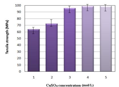
Fig. 3. Tensile strength of net chitosan films, and chitosan films with different concentration of CuSO<sub>4</sub>.
