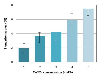
Fig. 4. Elongation at break for net chitosan films, and chitosan films with different concentration of CuSO<sub>4</sub>
