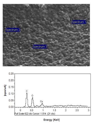
Fig. 2. Scanning electron microscopy micrograph and related EDX analysis for prepared CuNPs/ Cts BNCs film.
