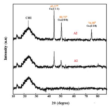
**Fig. 1.** Powder X-ray diffraction patterns of chitosan and copper/chitosan BNCs for determination of copper crystals at different CuSO<sub>4</sub> concentrations: (A1) 0.06mol/L, (A2) 0.15mol/L.
