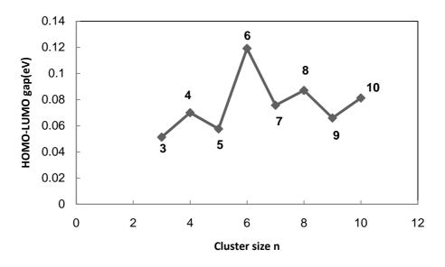
Fig.3. Size dependence of the HOMO-LUMO energy gaps for the Cu<sub>n</sub> clusters.
