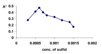
**Fig.4.** Effect of sulfide concentration. Conditions: pH, 4.2, lauth's violet5.4 10-5M,100 ng/ml Te(IV),at30<sup>°</sup>C.
