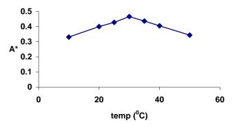
**Fig.5.** Effect of temperature on reaction. Conditions: pH, 4.2, lauth's violet 5.4 10-5 M, Sulfide6.0 10-4 M, 100 ng/ml Te(IV).
