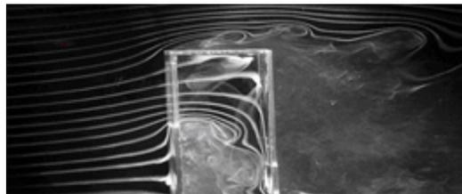
Fig.11: Visualized flow pattern inside and around the one-sided wind-catcher with flat roof
