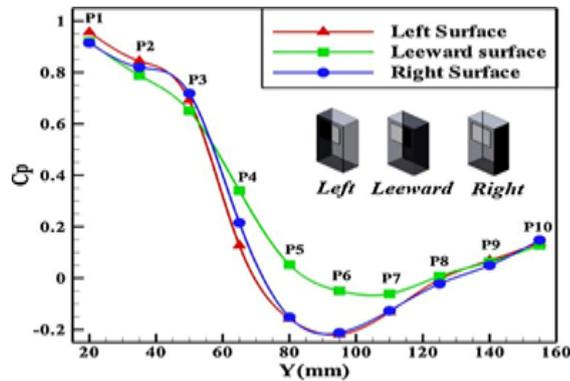
Fig. 12: Pressure coefficients on internal surfaces of the flat roof wind-catcher's channel at zero angle of incident
