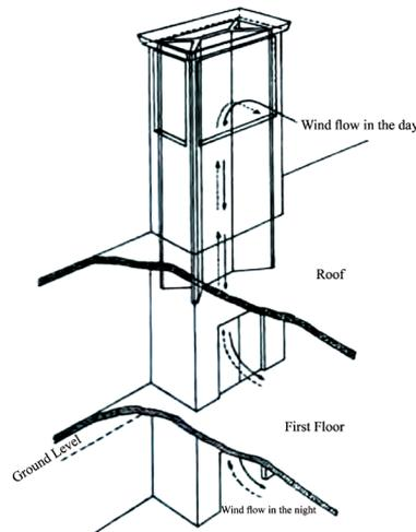
Fig. 3: Section of traditional windcatcher, the arrows shows the direction of the wind in day and night
