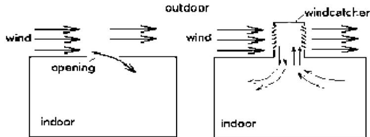
Fig. 1: Comparison of different ventilated rooms. (a) Rooms without windcatcher; (b) Rooms with windcatcher (Source: Li & Mak, 2007)
