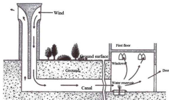
Fig. 4: Section of a wind catcher in Bam-Iran, the function of a windcatcher in blowing of the wind
