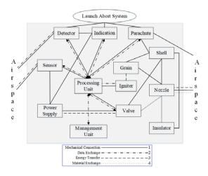
Fig. 6. System FMEA Block Diagram All-Space Of LAS
