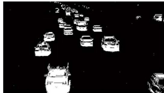
Fig. 4. Binary image obtained from the difference (after the thresholding)
