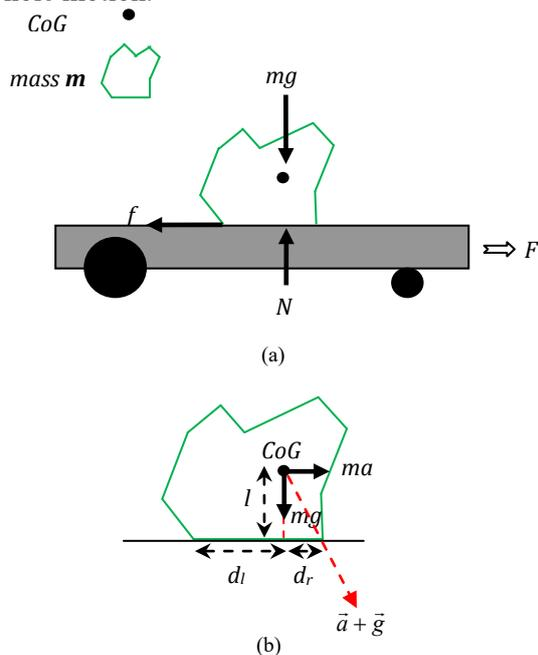
Fig. 1. (a) Manipulation task, (b) free diagram of the object.
