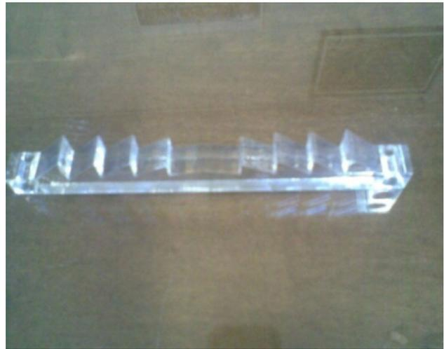
**Fig. 3** A single semi-Fresnel lens
