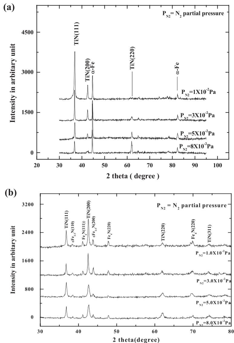
**Figure 6** Variation of XRD of TiN with nitrogen partial pressure. (a) Bare substrate and (b) plasma-nitrided substrate.
