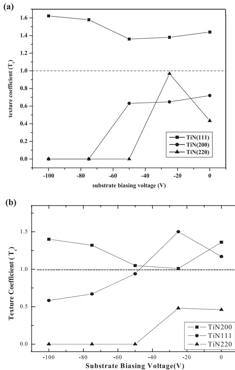
**Figure 9** Variation of  $T_c$  of TiN planes with substrate biasing voltage. (a) Bare substrate and (b) plasma-nitrided substrate.
