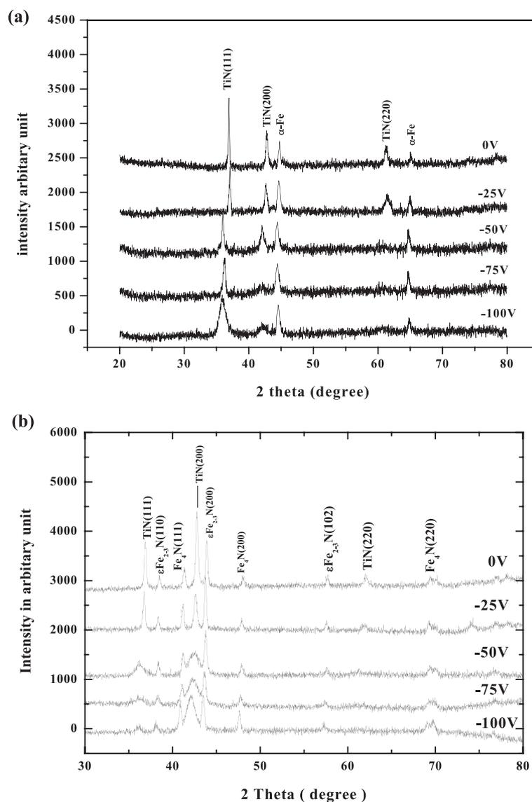
**Figure 7** Variation of XRD of TiN with substrate biasing voltage. (a) Bare substrate and (b) plasma-nitrided substrate.
