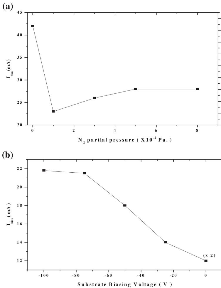
**Figure 4**  $I_{bias}$  as a function of (a)  $N_2$  partial pressure and (b) substrate biasing voltage.
