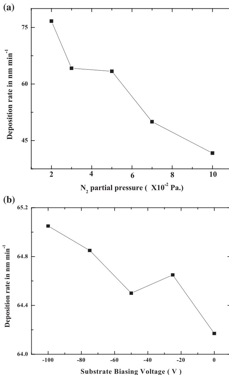
**Figure 5** Deposition rate as a function of (a)  $\text{N}_2$  partial pressure and (b) substrate biasing voltage.
