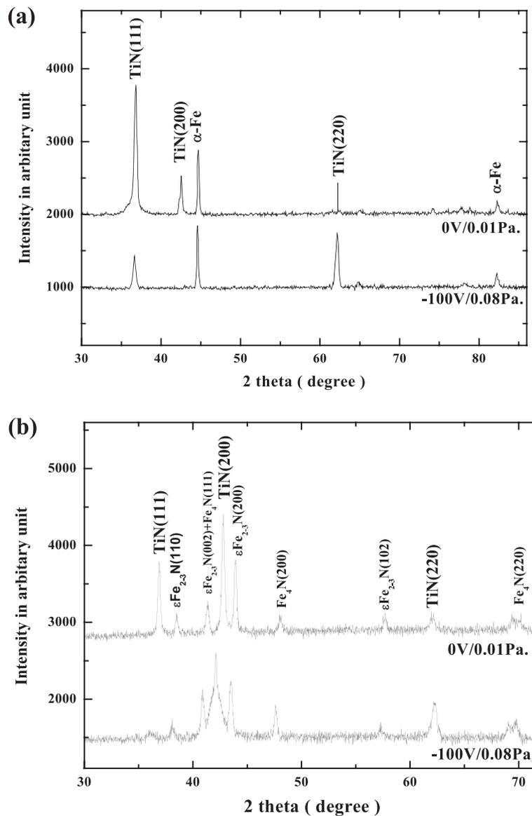
**Figure 10** Variation of XRD of TiN. (a) Bare substrate and (b) plasma-nitrided substrate at extreme ion bombardment condition.
