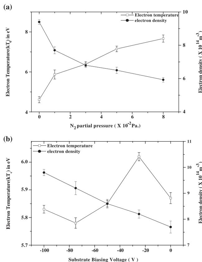
**Figure 2** Variation of  $N_e$  and  $T_e$  with (a)  $N_2$  partial pressure and (b) substrate biasing voltage.
