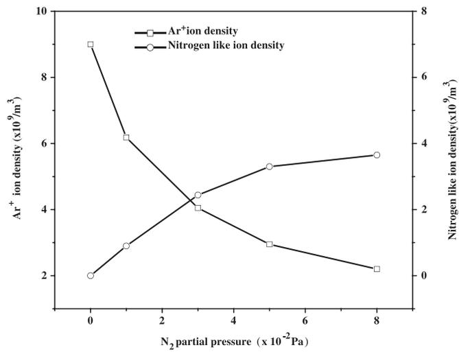
**Figure 3** Effect of nitrogen partial pressure on density of  $Ar^+$  and nitrogen-like ions.
