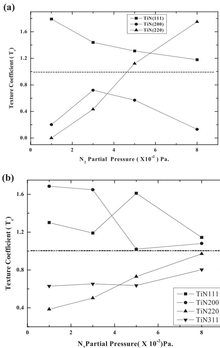
**Figure 8** Variation of  $T_c$  of TiN planes with nitrogen partial pressure. (a) Bare substrate and (b) plasma-nitrided substrate.
