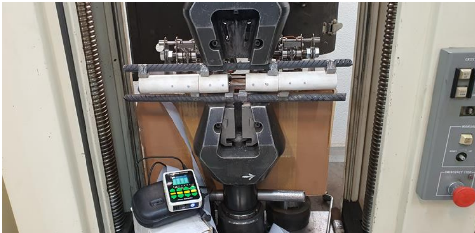
Figure 10. Bending force applied on four pieces of bone fixed in dynamic mode
