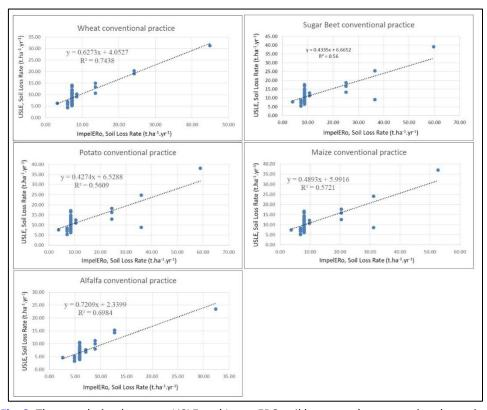
Fig. 8. The correlation between USLE and ImperERO soil loss rates by conventional practice
