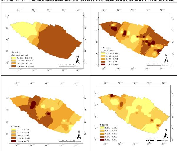
Fig. 2. Factor maps of rain erosivity, soil erodibility, slope length and slope steepness in the study area
