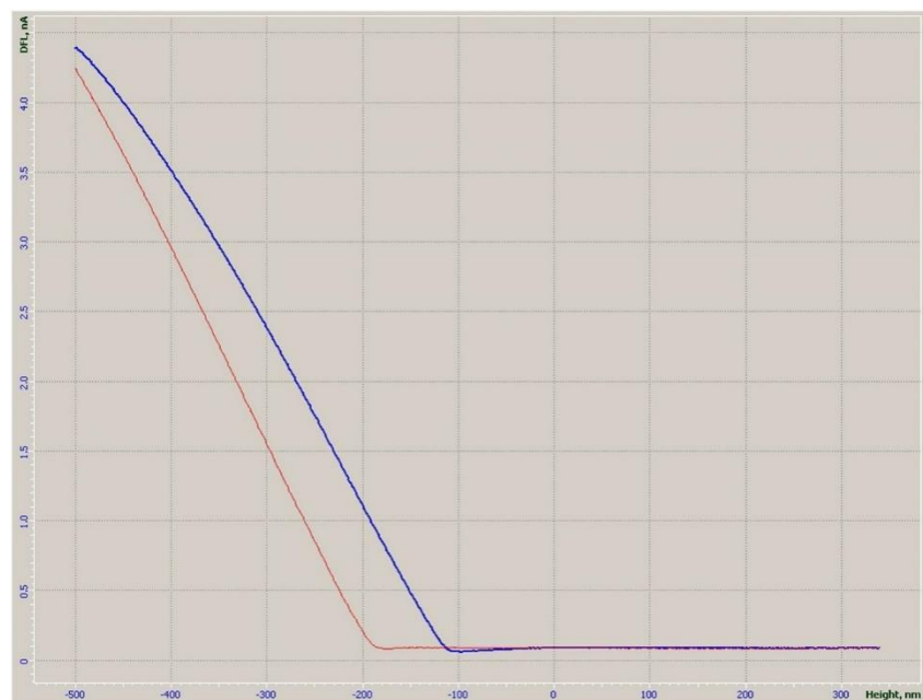
Figure 5. Average vertical deflection of the AFM cantilever versus (piezoelectric) movement for 20 indents for polystyrene (PS) sample by NT-MDT SOLVER P47 scanning probe microscope
