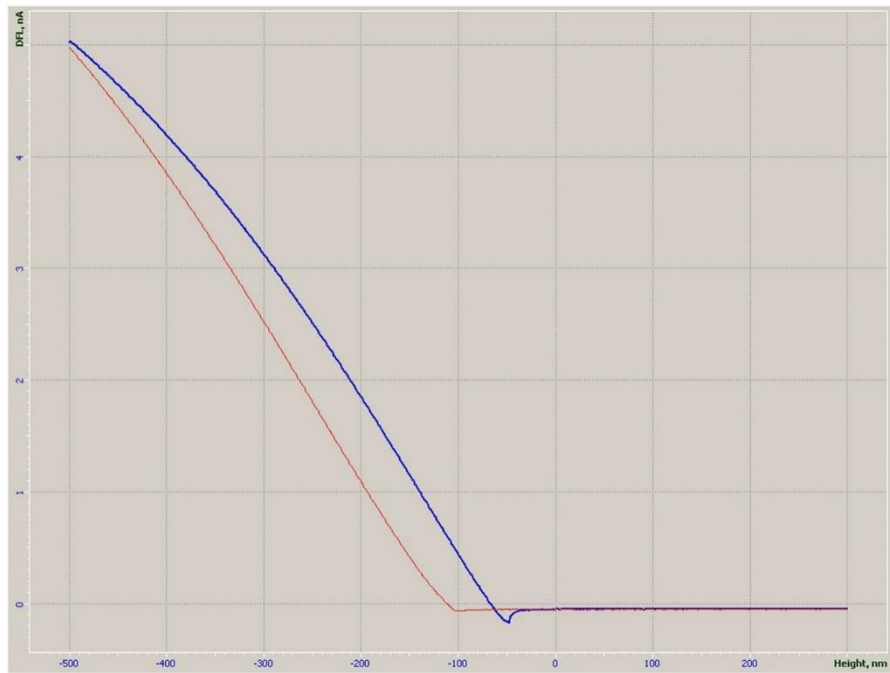
Figure 6. Average vertical deflection of the AFM cantilever versus (piezoelectric) movement for 20 indents for polypropylene (PP) sample by NT-MDT SOLVER P47 scanning probe microscope
