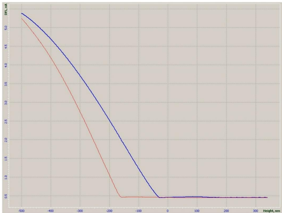
Figure 7. Average vertical deflection of the AFM cantilever versus (piezoelectric) movement for 20 indents for polycarbonate (PC) sample by NT-MDT SOLVER P47 scanning probe microscope
