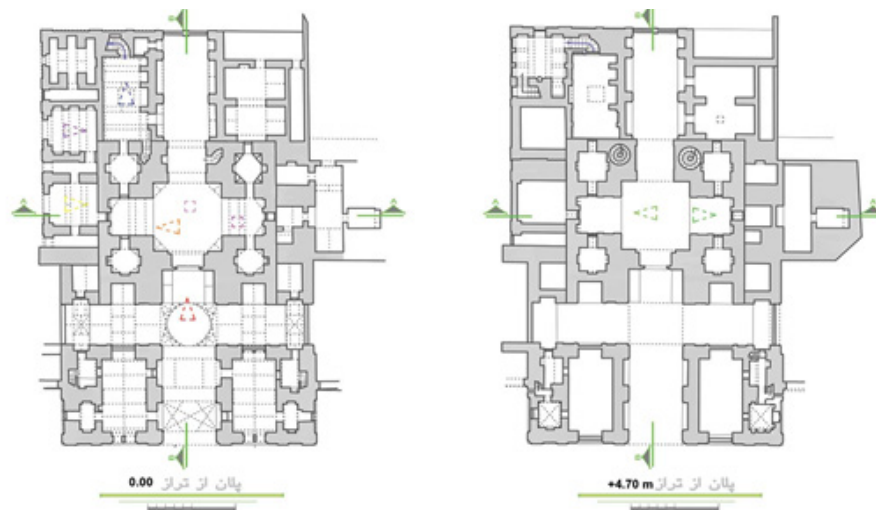
Fig. 6: Plan–elevation pair revealing the internal network of courts, corridors, and loggias that sustain controlled circulation and microclimatic moderation while projecting a disciplined public façade toward the square.
