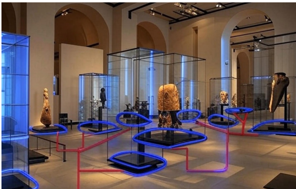
Fig 10. Schematic of FOS protection in the Louvre Museum sample area in Paris, where blue fiber optic cables are placed on the surface and directly exposed to acoustic waves from disturbing agents, while gray cables are buried underground, where strain changes are minimal and negligible compared to those in cables located around ancient objects.
