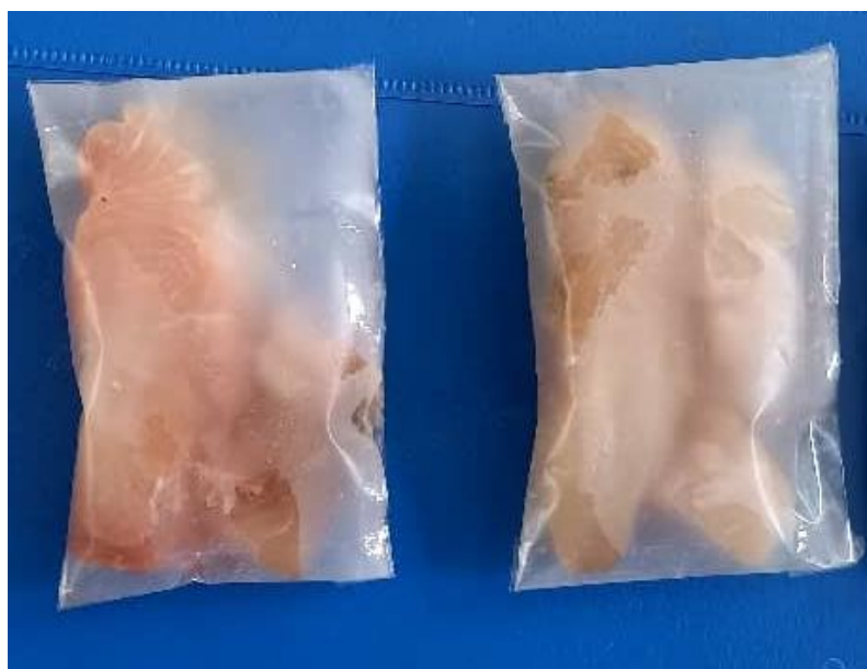
Fig. 2. Packaging of fish fillets in bilayer film integrated with RChNPs.
