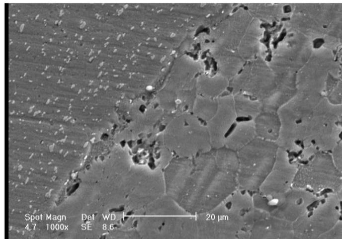
Figure 9. The microstructure of Stir zone (left) with small precipitates and HAZ (right) with bigger grains and precipitates
