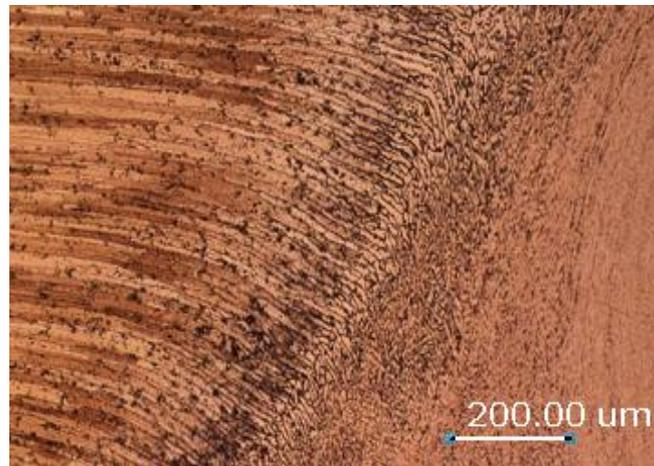
Figure 10. The deformed grains in the TMAZ
