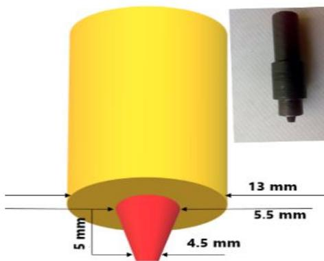
Figure 3. The FSP tool used in the present study
