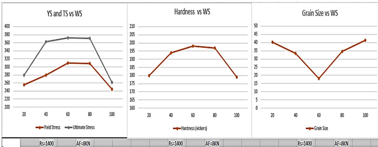
Figure 12. Welding Speed effect on mechanical properties at constant Rotational Speeds of 1400 based on Rajakumar et al. data on bulk 7075 Al Alloy
