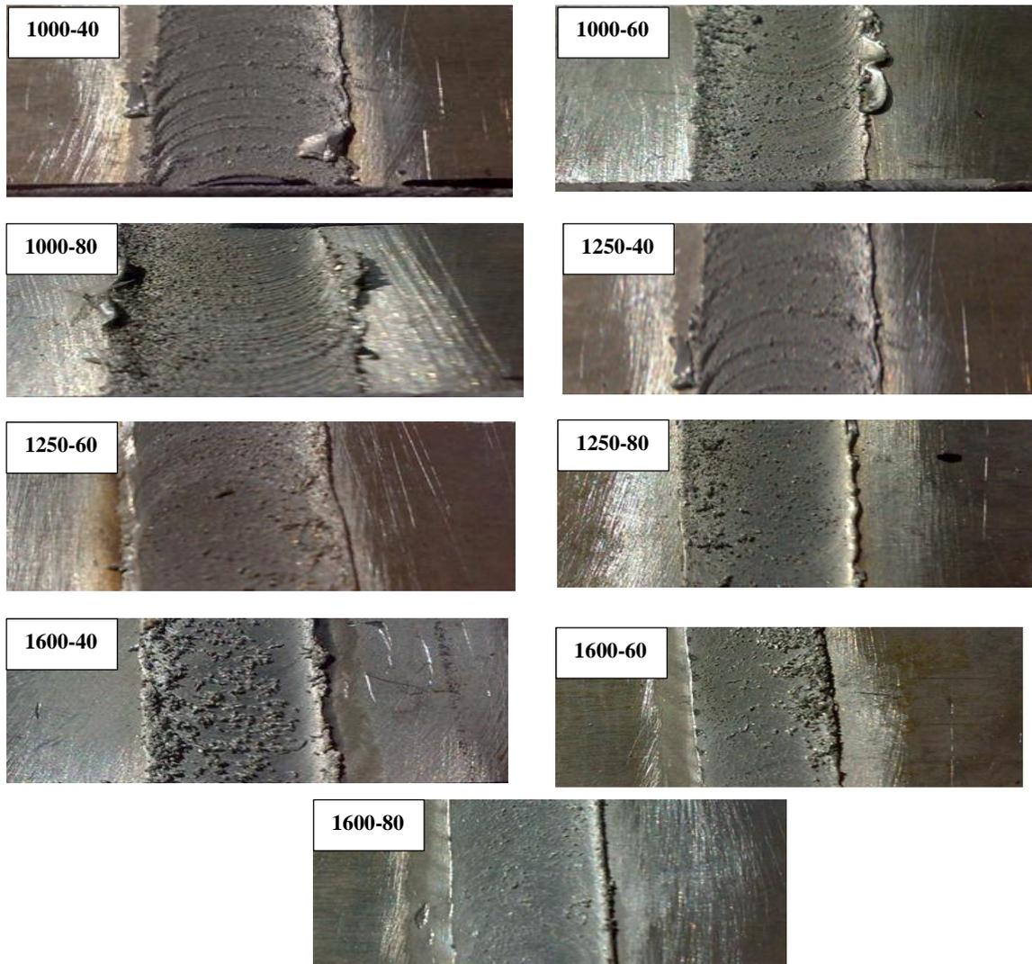
Figure 5. Optical micrographs of friction stir processed samples after the first pass with different RS and WS
