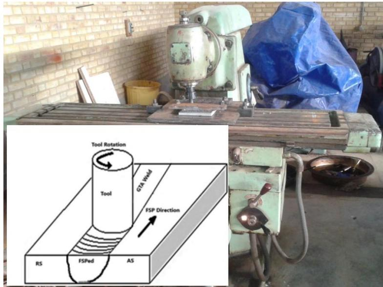
Figure 2. Vertical milling machine and schematic drawing of FSP
