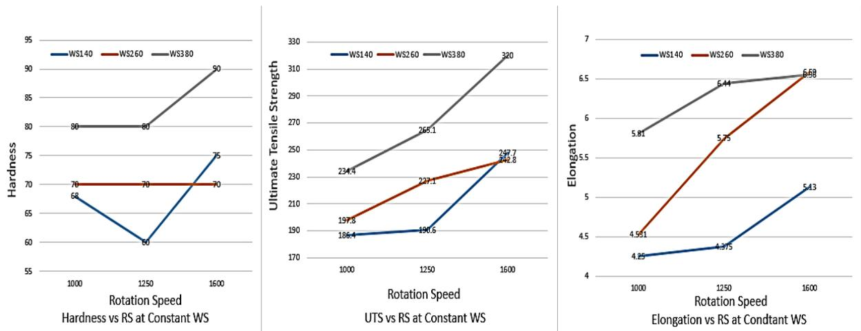
Figure 13. Rotational Speed effect on mechanical properties at constant Welding Speeds on 7075 Al Alloy joined by GTAW
