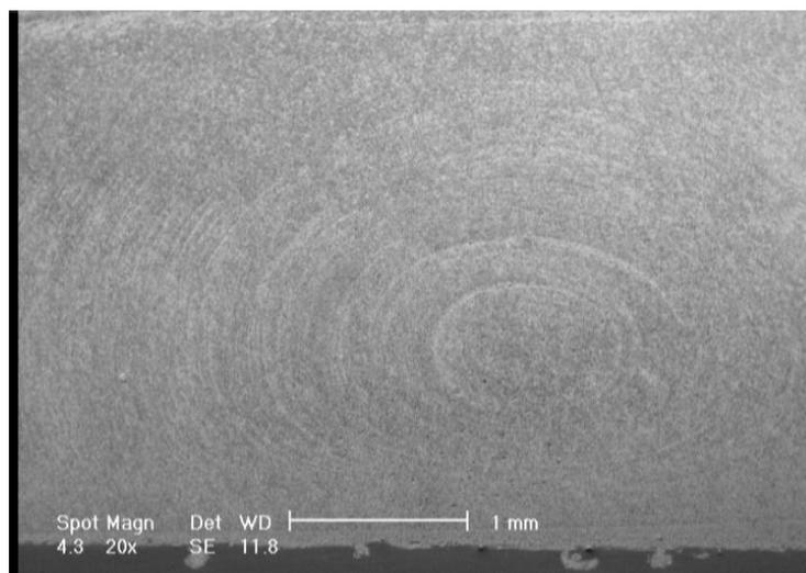
Figure 6. The elliptical 'onion' structure in the center weld
