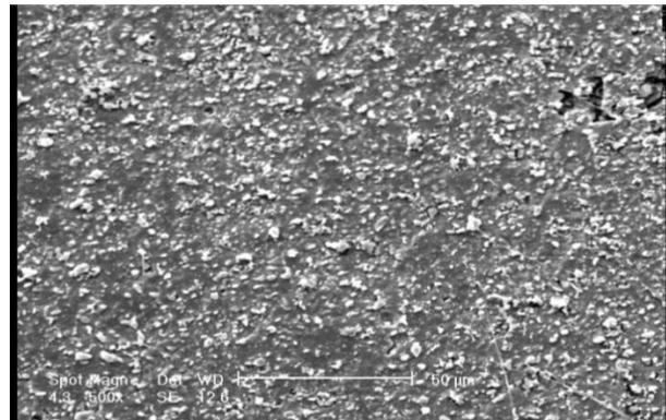
Figure 8. SEM micrographs of nugget zone in FSP weld
