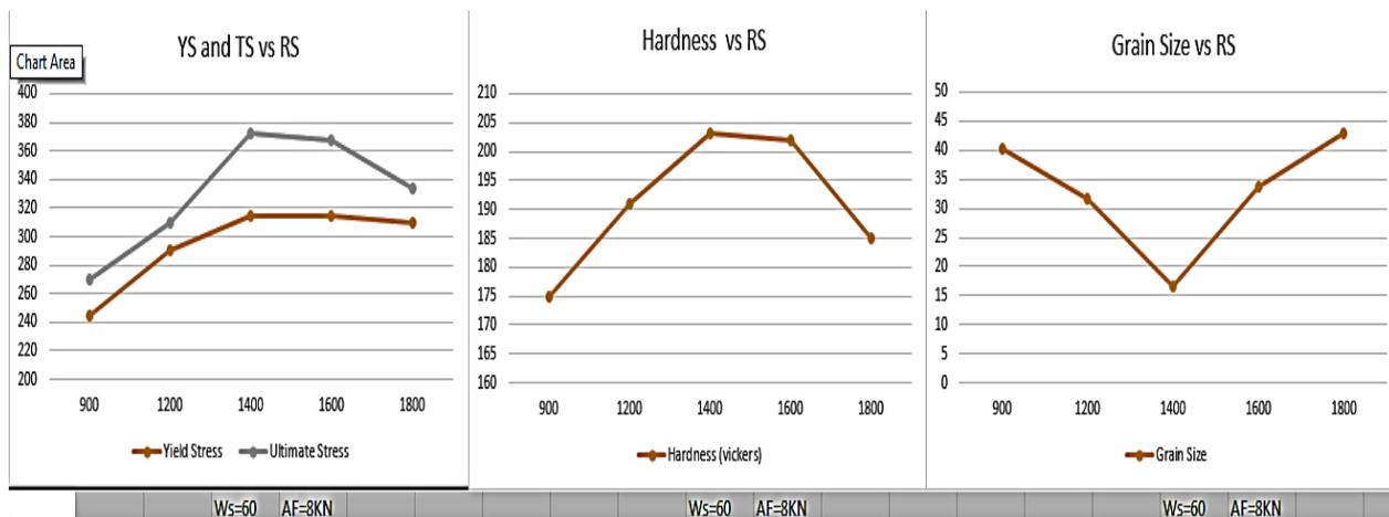
Figure 14. Rotational Speed effect on mechanical properties at constant Welding Speed of 60 based on Rajakumar data on bulk 7075 Al Alloy
