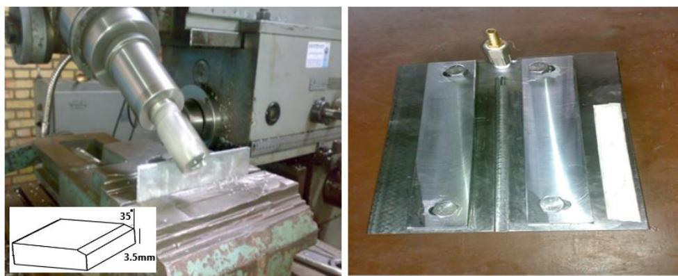
Figure 1. Preparing spacers for GTA welding
