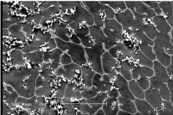
Figure 7. SEM micrographs of unprocessed weld
